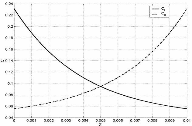
**Figure 3.** Diffusion fields of converging interfaces, Al-4Cu system,  $\Delta = 0.01$  cm.
