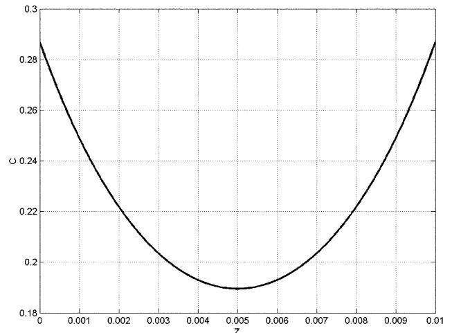
**Figure 4.** Resultant diffusion field, Al-4Cu system,  $\Delta = 0.01$  cm.
