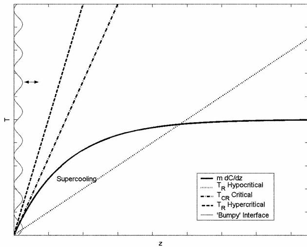
**Figure 2.** Condition for shape instability and stability as per constitutional supercooling.
