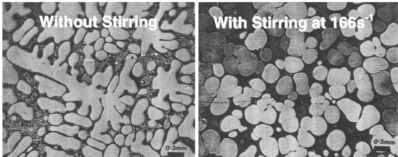
**Figure 1.** Al-1.5wt.%Cu cooled at  $40^{\circ}\text{C min}^{-1}$  from above the liquidus to  $588^{\circ}\text{C}$  and held isothermally for 3 h before quenching (Doherty 1982).
