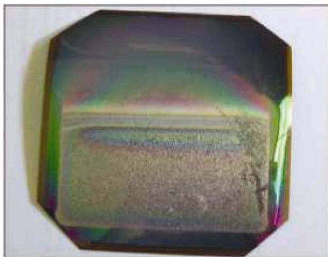
Figure 2. Back reflector on Upilex-S with a -Si triple cell on bottom, showing peeling.
