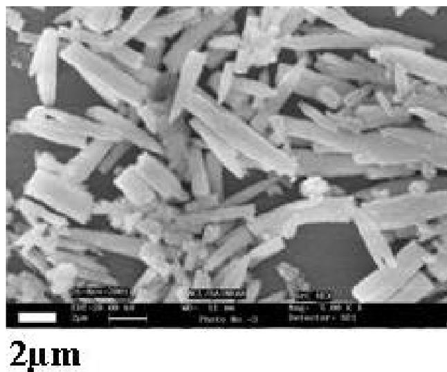
**Figure 4.** SEM image of  $\text{SrCO}_3$  crystals grown in a biphasic mixture of chloroform (without ionizable surfactant) and water in the control experiment.
