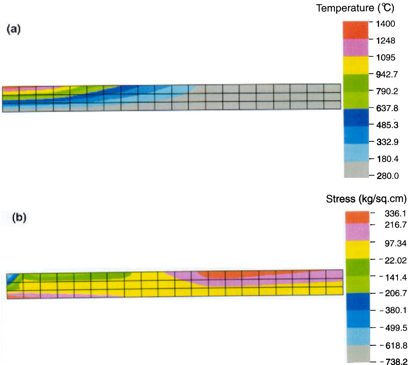
**Figure 3.** (a) Temperature and (b) thermal stress distribution in an axis-symmetric plane of solid cordierite body corresponding to a maximum temperature of 1400°C at the centre of top surface as calculated by FEM.
