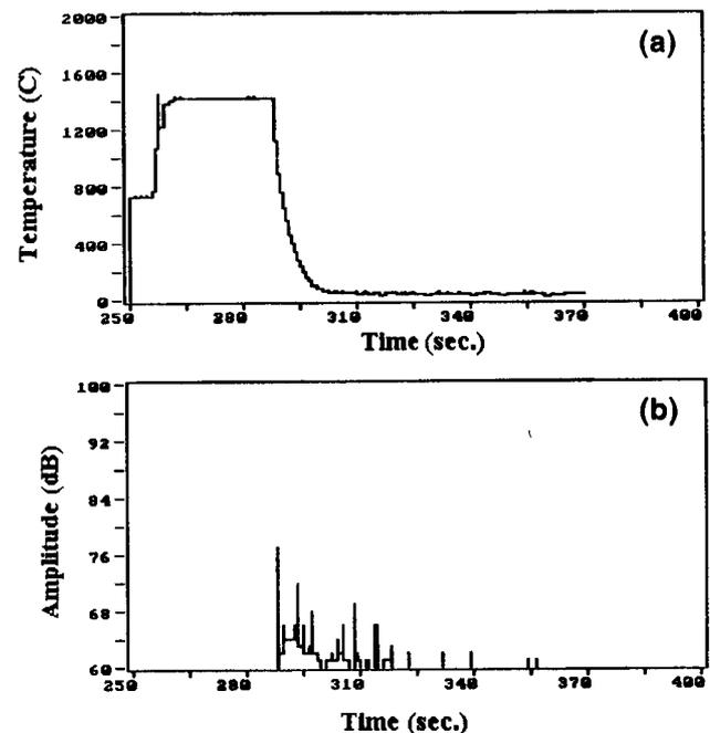
**Figure 2.** (a) Temperature profile of the hot zone and (b) acoustic emission signals of the cordierite honeycomb (400 cpsi) recorded during thermal shock test.
