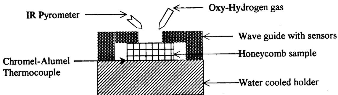
Figure 1. A close view of the sample with oxy-hydrogen flame heating during the thermal shock test.
