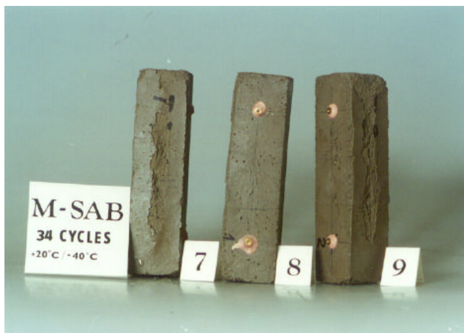
Figure 3. Surface damage of M-SAB mortar specimens subjected to FTC.
