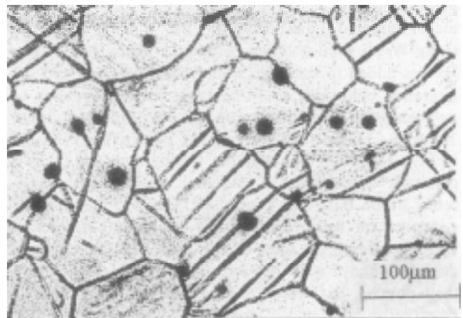
Figure 2. Microstructure of the alloy after 2 h at 250°C with 5 MPa stress (parallel boundaries, i.e. parallel to the stress axis in the sample).
