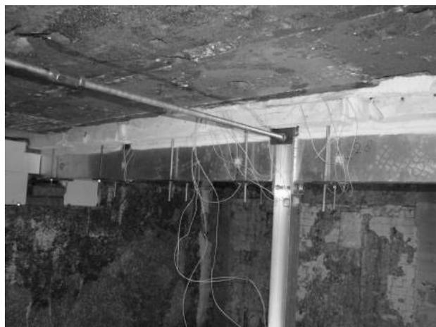
Figure 8. Insulation on top of the specimens for the tests at elevated temperature
