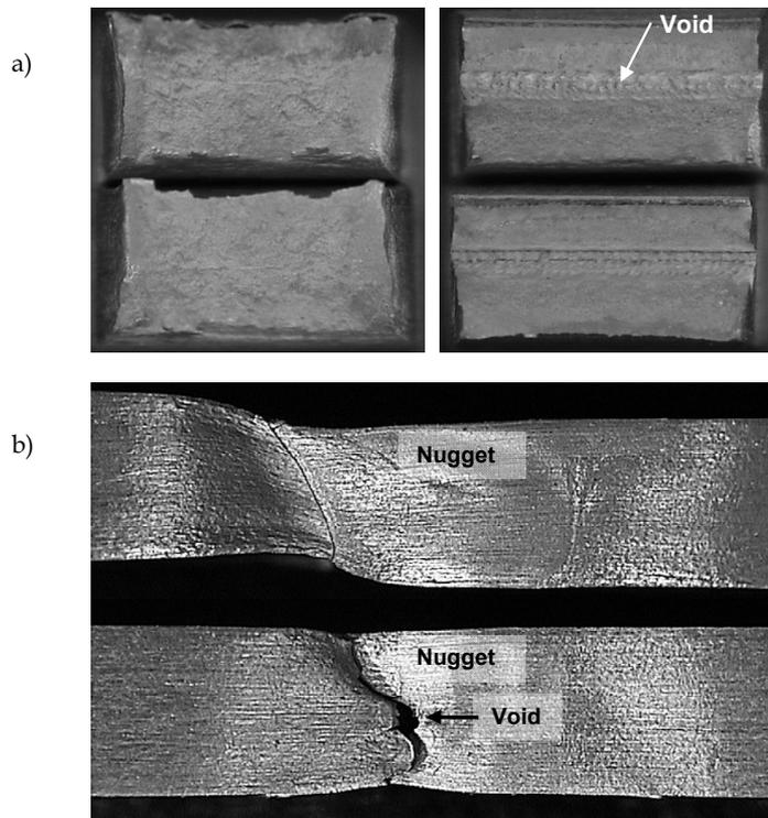
*Figure 5: Fracture surfaces a) and side views b) of tensile test specimens with friction stir welds in aluminium alloy AA6061-T6. The void-free specimen failed in the heat-affected zone while the specimen with a running void failed inside the weld nugget.*
