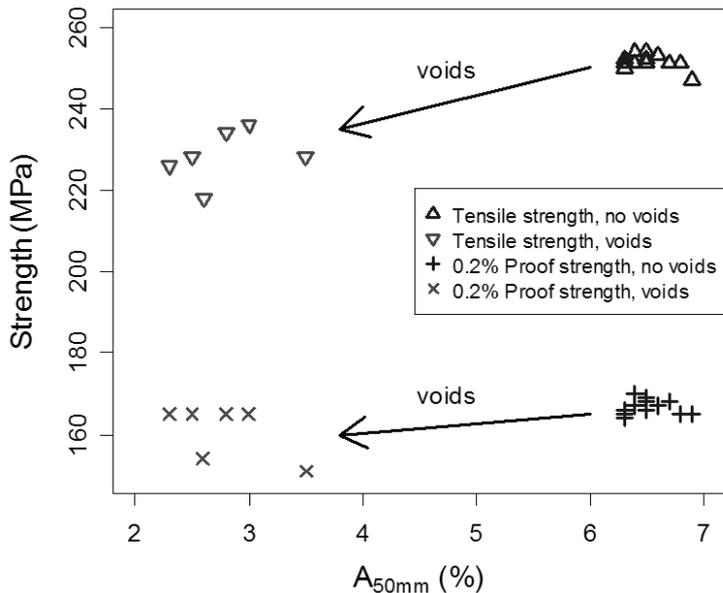
Figure 4: Influence of voids on proof strength, tensile strength, and elongation to fracture of friction stir welds in AA6061-T6
