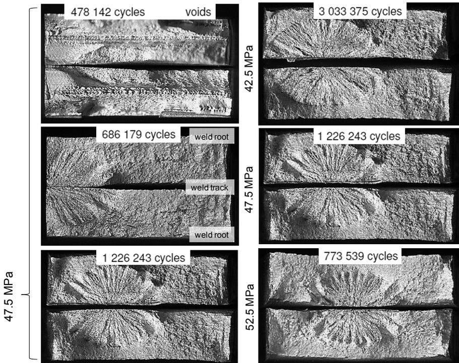
Figure 7: Fracture surfaces of fatigue test specimens with friction stir welds in aluminium alloy AA6061-T6. The images on the left depict different types of fracture that occurred in specimens tested at the same stress amplitude. The images on the right demonstrate that the area of the fatigue fracture surface decreases as the stress amplitude increases.
