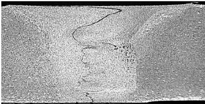
Figure 3: Cross section of friction stir weld in aluminium alloy AA6061-T6 after etching in caustic soda. The dark line corresponds to a band of small, finely distributed oxide particles of approximately  $1\ \mu\text{m}$  in diameter.
