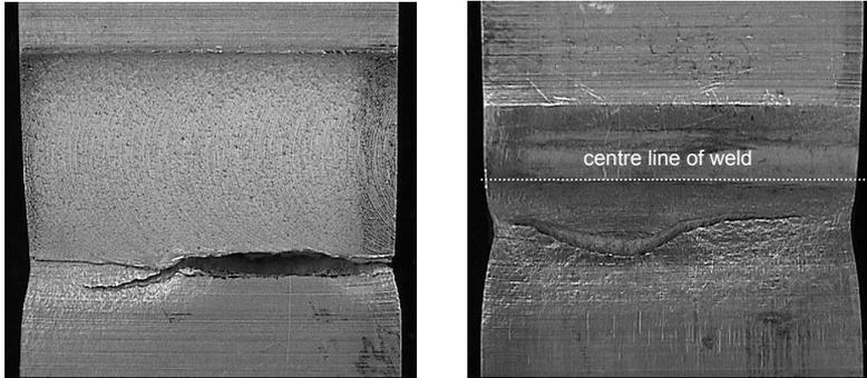
Figure 8: Top and bottom view of the crack of a specimen cycled at a stress amplitude of 47.5 MPa for 1 226 243 cycles until fracture occurred. The crack nucleated at the edge of the weld track on the advancing side of the friction stir weld.
