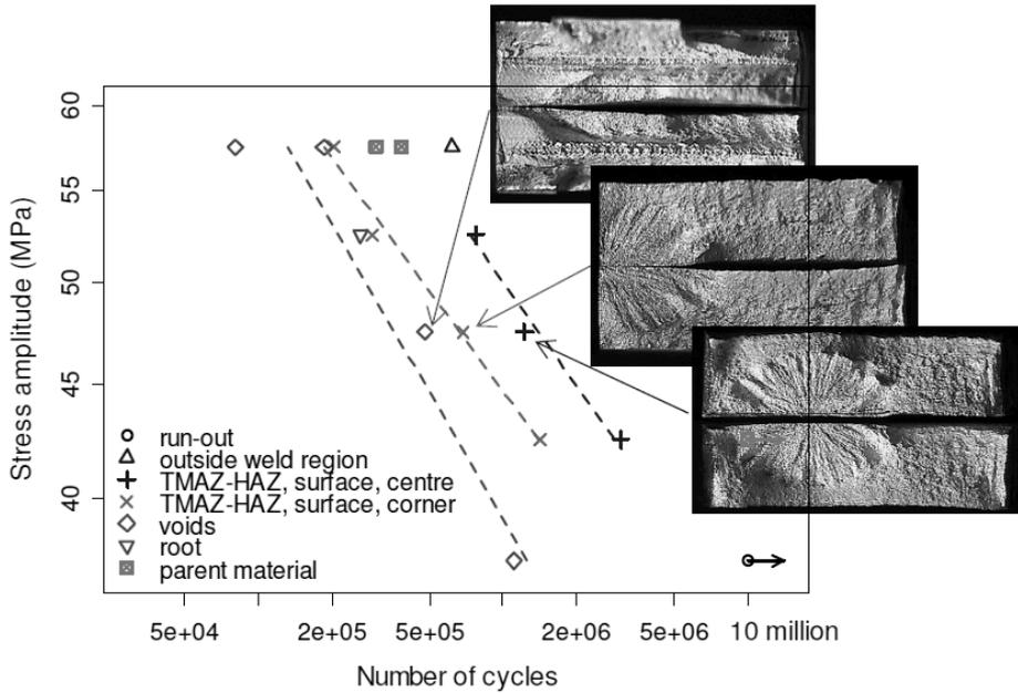
Figure 6: Stress amplitude-fatigue life data for friction stir welds in aluminium alloy AA6061-T6. Power-law lines were fitted to those specimens that had the same type of crack nucleation and growth. Locations of crack nucleation, or other information on the specimens, are given in the legend. Fracture surfaces of three selected specimens are also shown.
