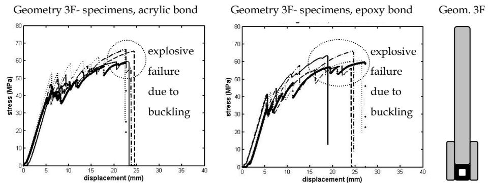
Figure 20: Stress-displacement diagrams of geometry 3F -specimens (for both adhesives).
