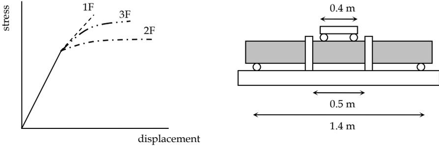
Figure 16: (left) Schematic stress-displacement diagram of the reinforcement geometries 1F, 2F and 3F.
