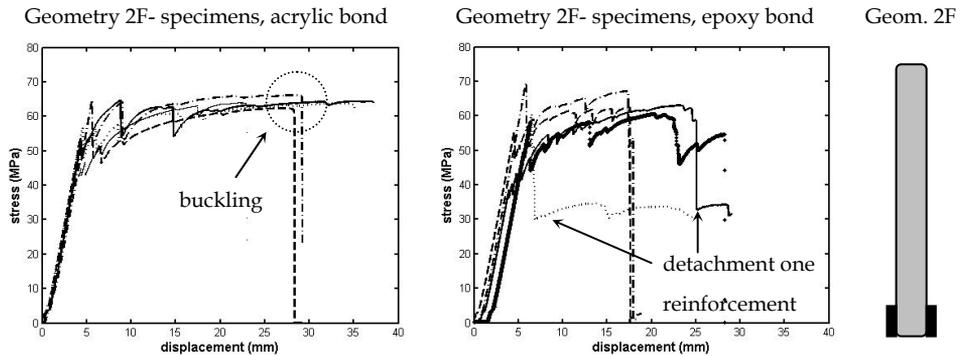
Figure 19: Stress-displacement diagrams of geometry 2F -specimens (for both adhesives).
