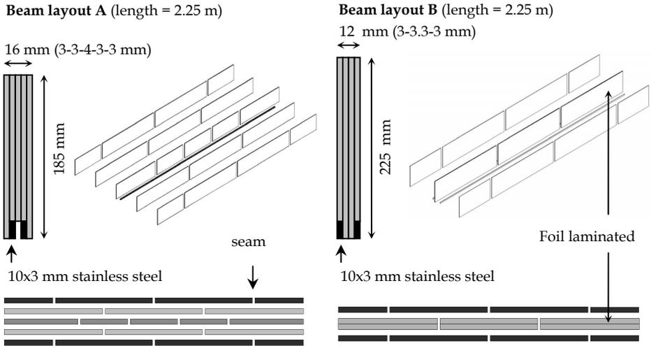
Figure 11: Schematic cross-section geometry and segmentation scheme of alternative beam designs.
