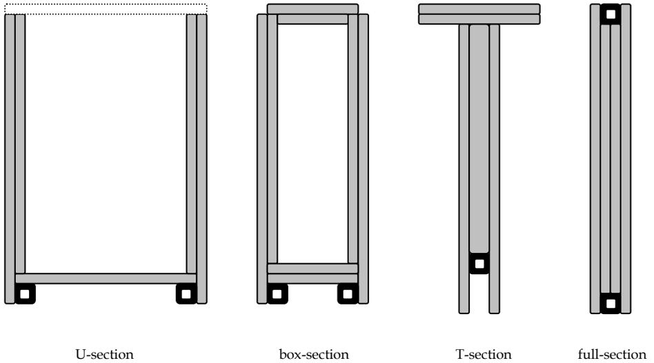
Figure 10: Alternative cross-section designs, developed at Delft University of Technology
