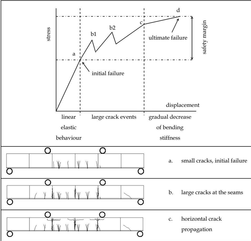
Figure 8: (up) Schematic stress-displacement diagram of bend tests on reinforced glass beams.
