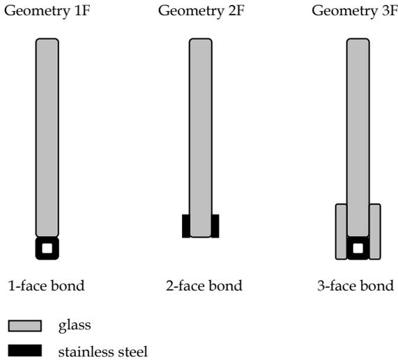
Figure 15: Alternative reinforcement geometries, which differ in 1-, 2- or 3-face bond.
