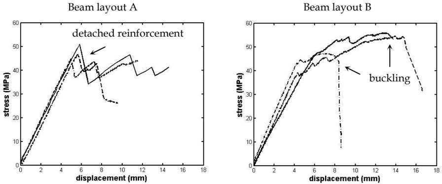
Figure 12: Stress-displacement diagrams of beam layout A-specimens and beam layout B-specimens.
