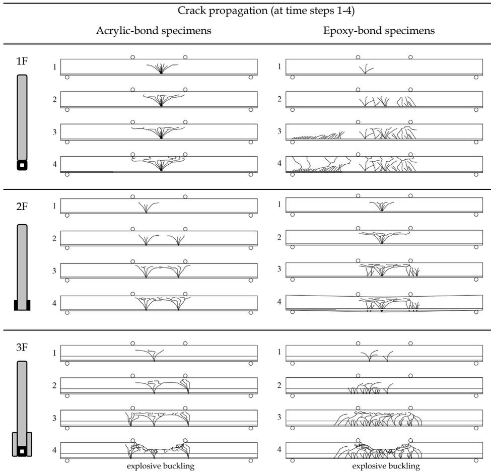
Figure 21: Schematic overview of crack propagation at different time steps (1-4) for both adhesives and all reinforcement geometries. (1 = initial failure 4 = ultimate failure)
