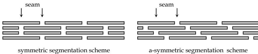
Figure 7: Examples of symmetric and a-symmetric segmentation scheme for a four-layer beam. (top view, figures are schematic and dimensions are without proportion)
