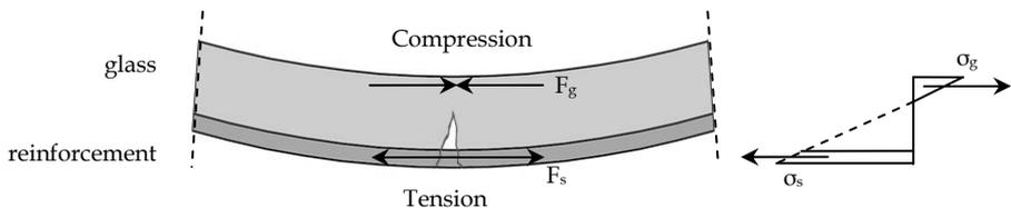
Figure 1: Schematic overview of distribution of forces after glass failure
