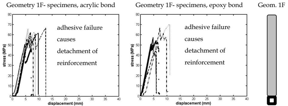
Figure 18: Stress-displacement diagrams of geometry 1F -specimens (for both adhesives).
