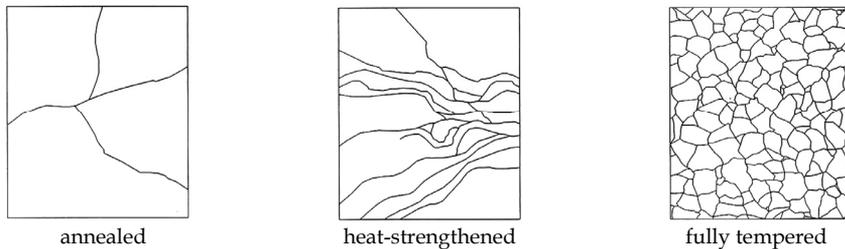
Figure 2: Fracture pattern of annealed, heat-strengthened and fully tempered float glass [Schittich, 1999]
