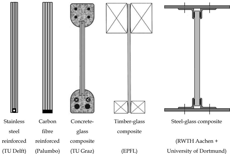
Figure 4: Similar structural glass composite beam concepts. The figures are schematic and not to the same scale
