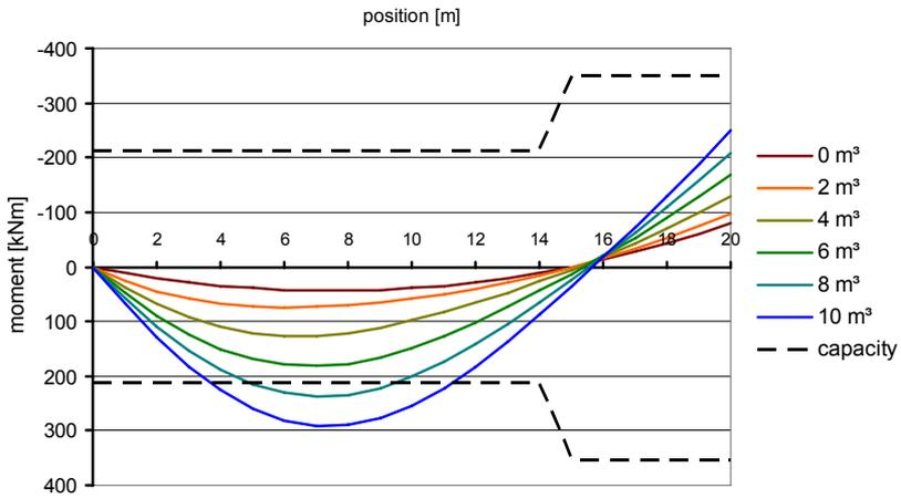
Figure 9: The bending moments in the beam as function of the volume of stored water
