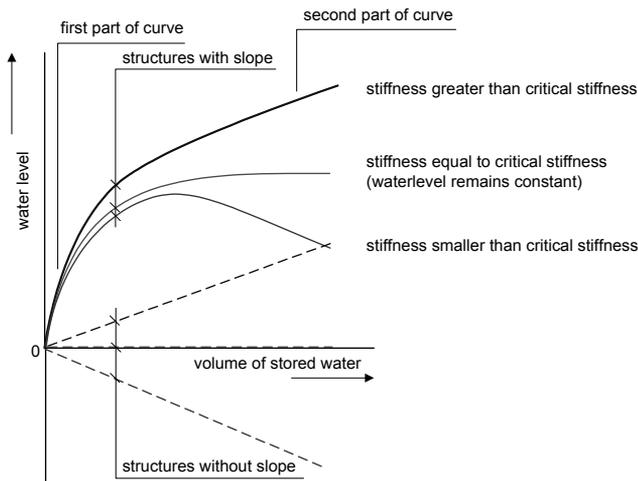
Figure 12: The relation between the water level and the volume of stored water for different stiffness
