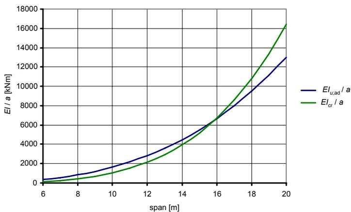
Figure 13: The relation the required stiffness for displacement requirements, the critical stiffness for ponding and the span by a simple span
