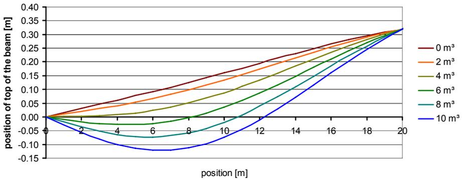
Figure 8: The deformed shape of the structure depending on the volumes of stored water
