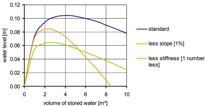
Figure 11: The relation between the water level and the volume of stored water for different situations
