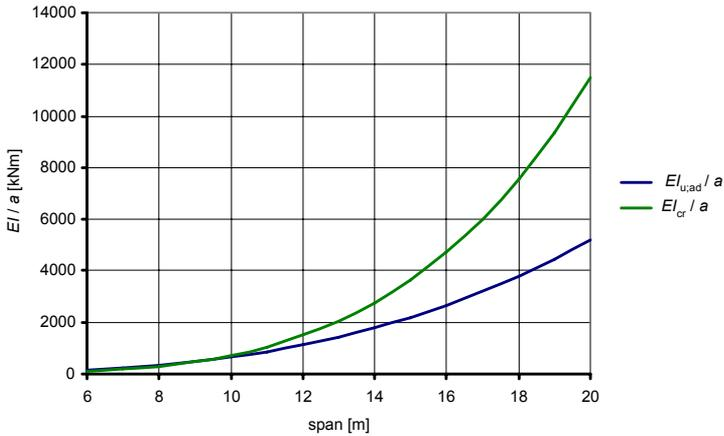
Figure 14: The relation the required stiffness for displacement requirements, the critical stiffness for ponding and the span by a two span beam
