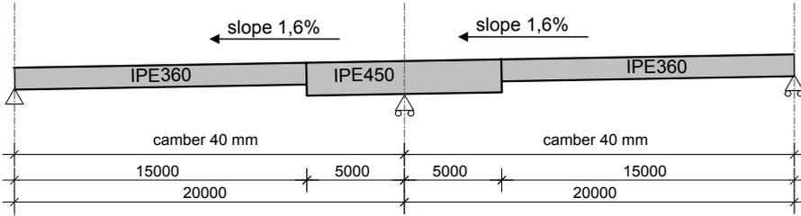
Figure 7: Structure considered, centre-to-centre-distance of adjacent beams is 5000 mm
