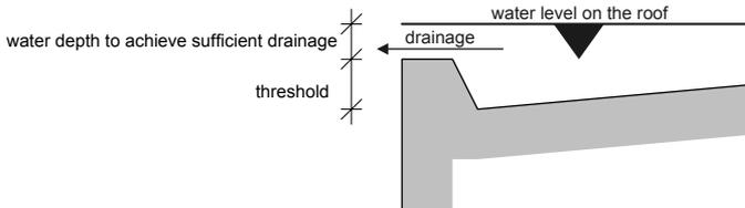
Figure 15: Overflow of emergency drainage system
