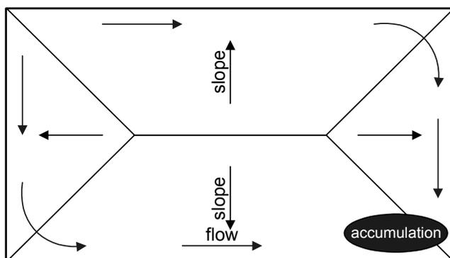
Figure 6: Flow of water on a roof to the area where accumulation takes place
