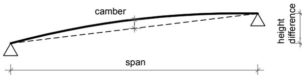
Figure 5: Slope caused by height difference and camber
