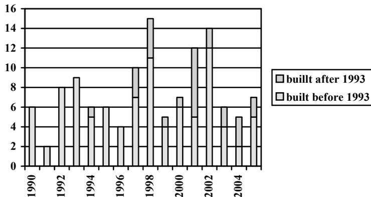
Figure 1: Number of light-weight flat roofs yearly collapsed in the Netherlands due to rainwater ponding. 50% of the total estimated. (Source: Hageman [1])
