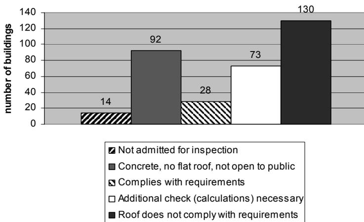
Figure 5: *Inspection results for objects with flat roofs*
