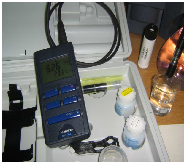
Figure 2. Determination of the oxygen content using the Oxi 315i equipment
