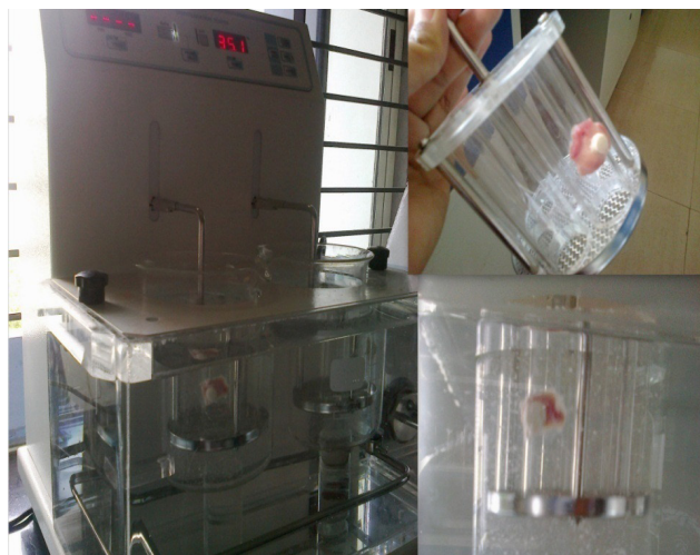
Figure 1: Modified disintegration apparatus for measurement of ex-vivo residence time
