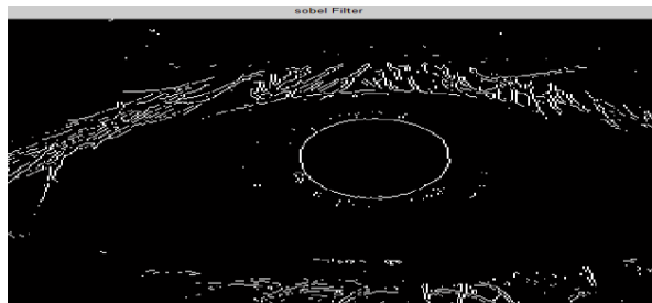
Fig.5.4 Detection of edges using Sobel mask.
