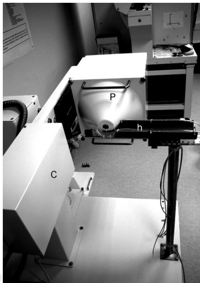
FIGURE 1. Close-up view of dedicated small-animal pinhole SPECT camera. P = pinhole collimator; C = counterweight; h = small-animal holder.
