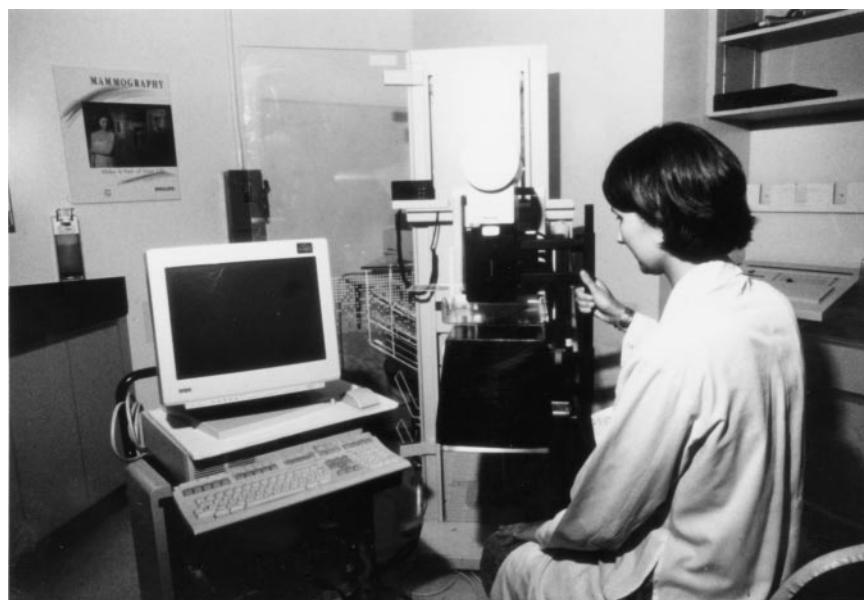
FIGURE 1. Photograph of PEM-1 system installed in mammography unit at Cedars' Breast Clinic. Lower detector is housed in standard mammographic magnification table and positioned below breast. Upper detector is positioned above compression paddle.
