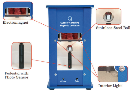
Fig. 1. Magnetic levitation system diagram
