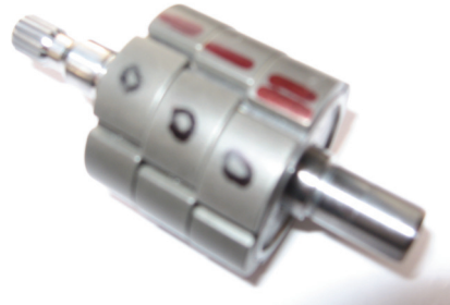
Fig. 11. Assembled rotor with 3 step-skew groups of 6 PMs
