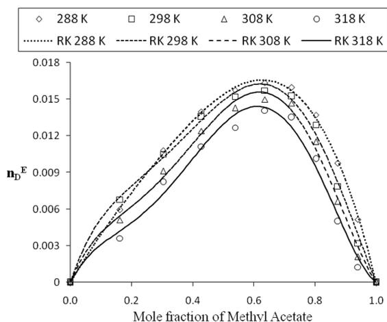
**Fig. 2.** Excess refractive index of Cyclohexane-Methyl Acetate binary system.
