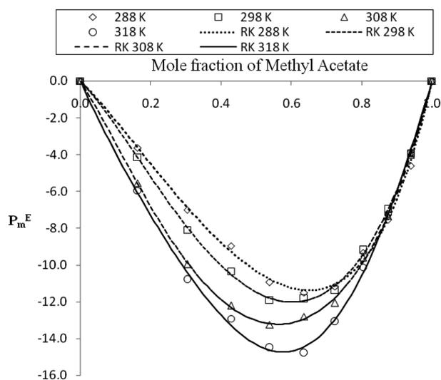
Fig. 5. Excess molar polarization of Cyclohexane-Methyl Acetate binary system.
