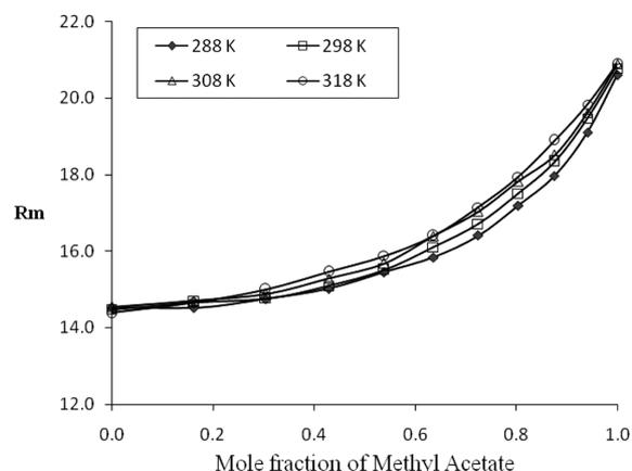
**Fig. 4.** Molar refraction of Cyclohexane-Methyl Acetate binary system.
