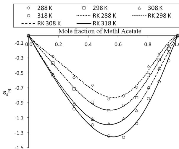
**Fig. 1.** Excess dielectric constant of Cyclohexane-Methyl Acetate system.
