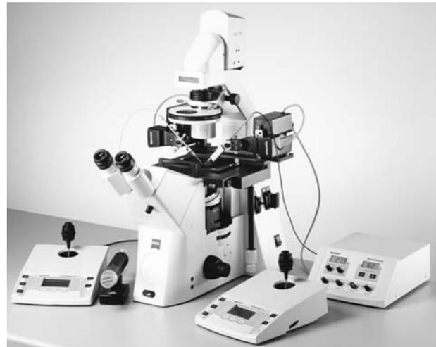
Figure 4. Photograph of the Piezo Power MicroDissector PPMD<sup>®</sup> System. The MicroChisel<sup>®</sup> is seen above the stage of a Zeiss inverted microscope on the right, while the NK2<sup>®</sup> Micromanipulator is on the left. Courtesy of Joel Lopez, Eppendorf USA.
