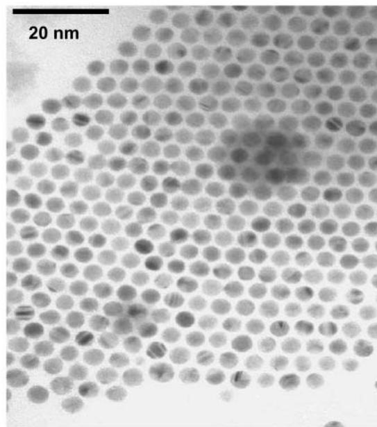
Figure 3. 2-D array of Au nanoparticles driven by capping agent of dodecanethiol on carbon film.
