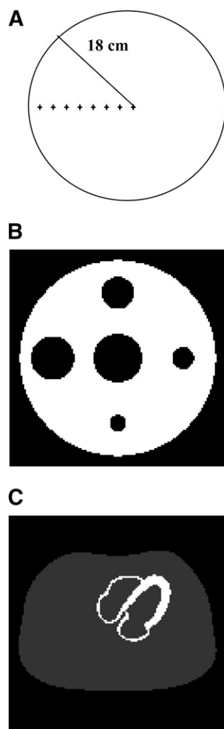
FIGURE 1. Computer simulations. (A) Uniform object used for 2D PSF estimations. Eight point sources with different locations are marked by plus signs. (B) Cold-lesion simulation. This object consists of 5 cylindric cold spots in uniformly attenuating cylinder of uniform activity. (C) Uniform cardiac simulation.
