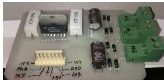
Fig. 6. H-Bridge Motor Control Circuit.
