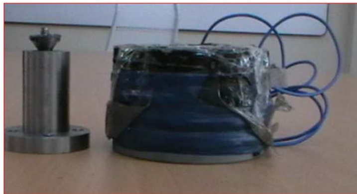
Fig. 3. Dissembled view of the MR Fluid Damper
