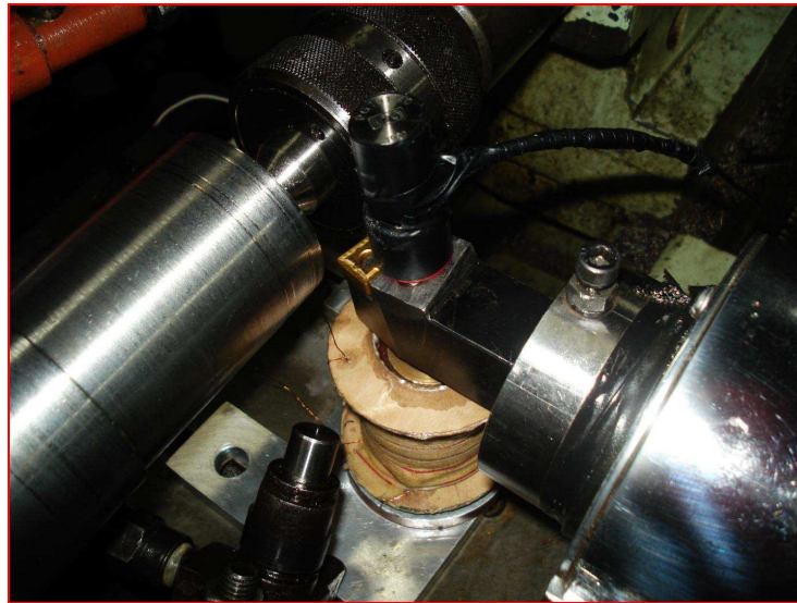
Fig. 2. Photograph of the experimental setup with MR fluid damper
