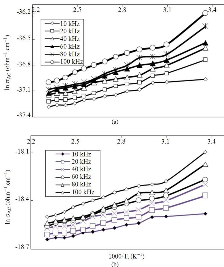
**Fig. 2.** Effect of temperature on AC-electrical conductivity (at different frequencies) for CNTs/PANI/Ag prepared by mixing method (a) and decoration method (b)
