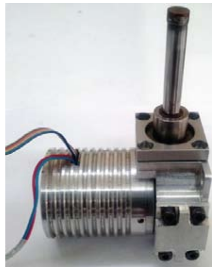
Figure 3. IDCA cryocooler prototype developed at SSPL.
