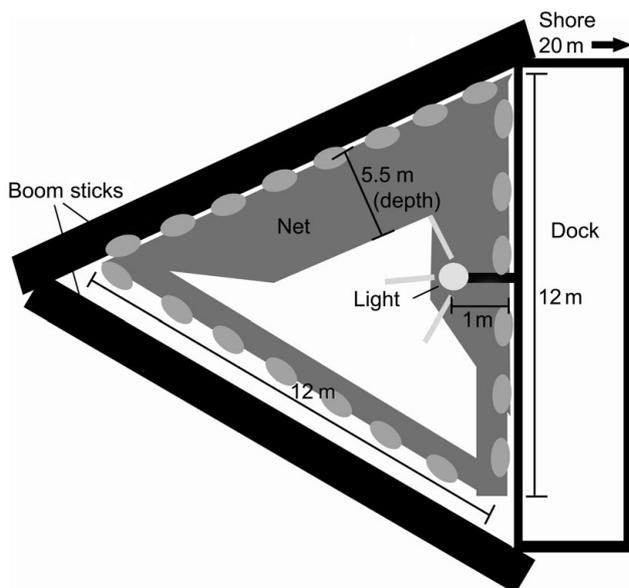
Fig. 1. Bird's eye view of experimental set up. Purse seine (dark grey): 5.5 m deep  $\times$  36.6 m long, arranged in a triangle against the dock and a boom stick frame (black). Half of the net was deployed (top half of the diagram), while the other half was cinched up at the surface of the water. The net hung essentially vertically; the perspective has been exaggerated to emphasize the deployment
