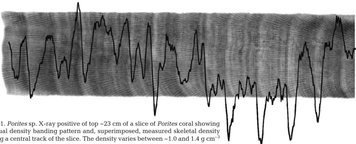
Fig. 1. *Porites* sp. X-ray positive of top ~23 cm of a slice of *Porites* coral showing annual density banding pattern and, superimposed, measured skeletal density along a central track of the slice. The density varies between ~1.0 and 1.4 g cm<sup>-3</sup>
