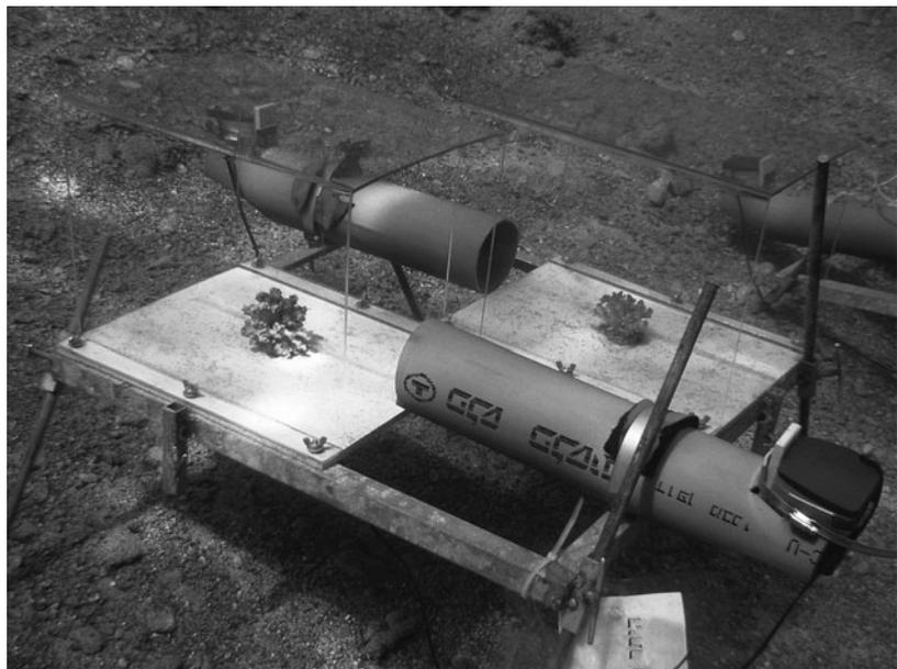
Fig. 1. Underwater setup of flow-manipulation experiment showing 2 units each consisting of a transparent, upside down U-shape box ( $40 \times 40 \times 30 \text{ cm}$ ) and a pump attached to a 50 cm long, 10.1 cm diameter pipe directed at the coral
