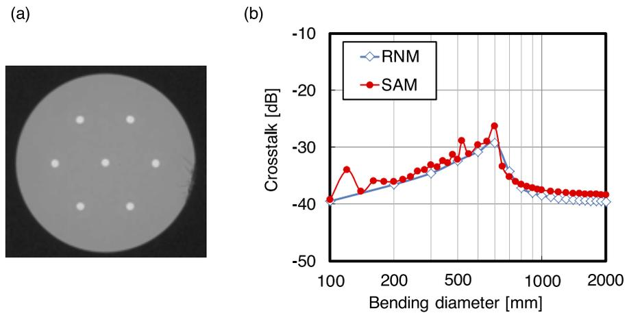
**Fig. 2.** Bending diameter dependence of crosstalk: (a) A cross sectional view of a fabricated MCF used for the measurement [5]. (b) Comparison of crosstalk between two simulation results.
