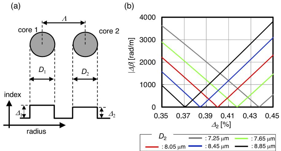
**Fig. 1.** Simulated absolute value of  $\Delta\beta$  as a function of  $D_2$  for different  $D_2$ : (a) Schematics of two-core model. (b) Simulation results.
