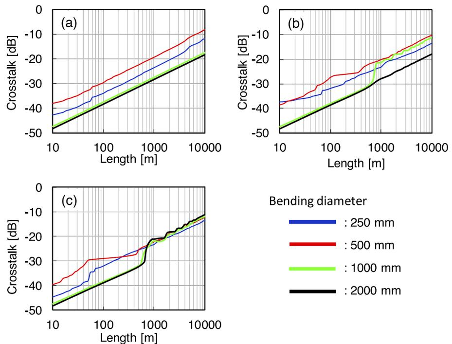
**Fig. 3.** Length dependence of crosstalk at 1550 nm for various  $A_{\Delta}$ : (a)  $A_{\Delta} = 0\%$  (No structural drift). (b)  $A_{\Delta} = 0.005\%$ . (c)  $A_{\Delta} = 0.01\%$ .
