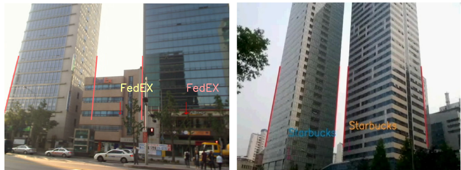
Fig. 5. Examples of 3DoF pose improvement results: pose improvement based on three vertical edges (left) and four vertical edges (right)
