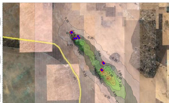
Fig. 13c: Isoleths plot for the maximum annual average ground level concentrations of methane in \mu\text{g m}^{-3}
