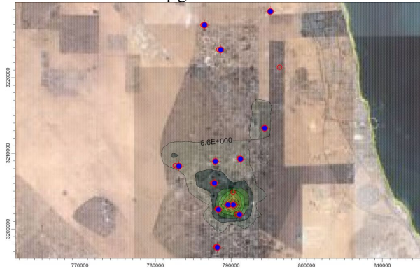
Fig. 11b: Isopleths plot for the maximum hourly average ground level concentrations of methane in \mu\text{g m}^{-3}
