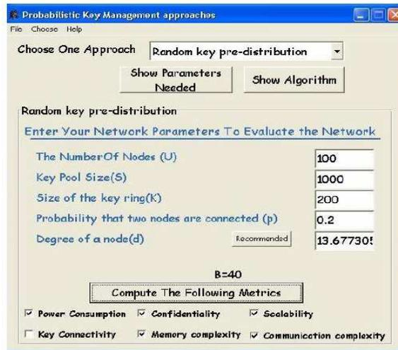
Fig. 7. Random Key pre-distribution and its parameters
