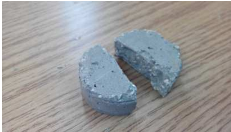
Fig. 3. Typical induced crack in a tested sample
