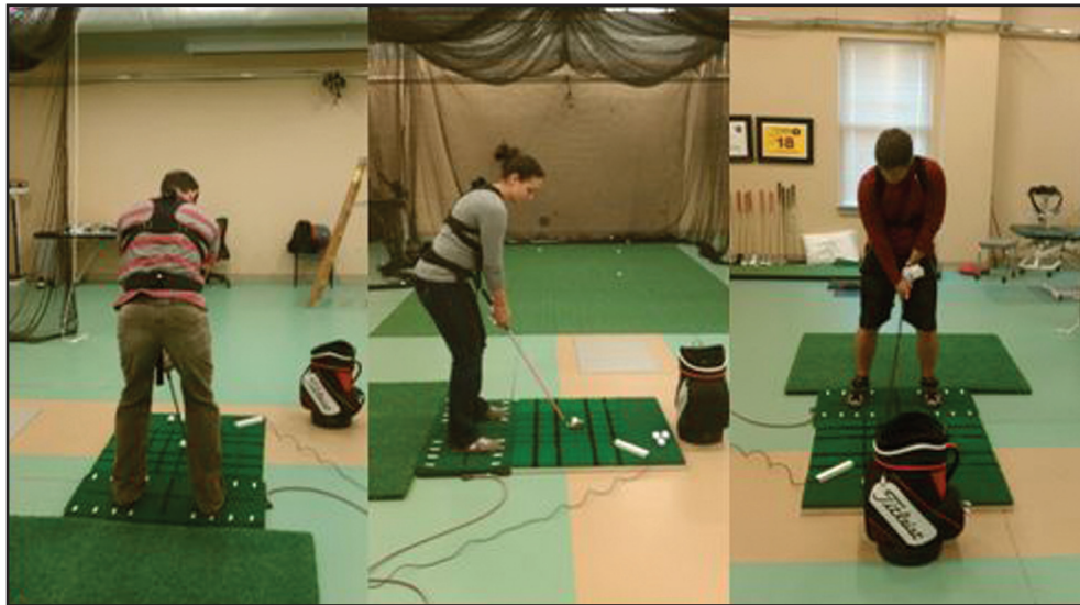
Figure 3. Subjects donned the K-vest equipment and were given 5 practice swings before data collection. The K-vest consists of 3 wireless motion tracking sensors: one on the sacrum, one between the scapulae and one on the glove of the lead wrist.
