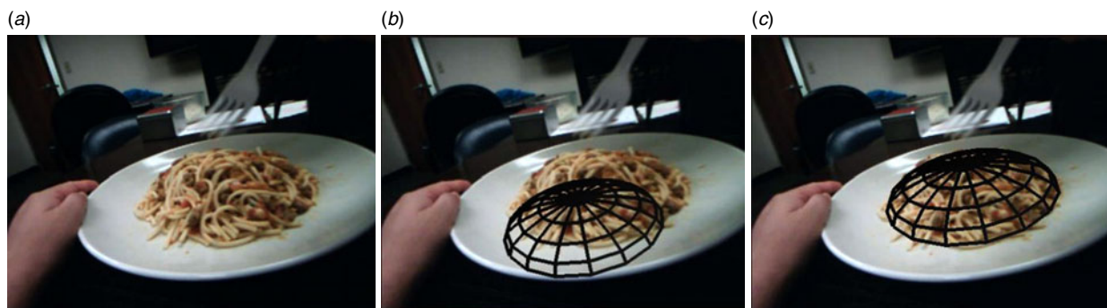
Fig. 2. (colour online) Spaghetti volume estimated using wire mesh: (a) spaghetti on plate, (b) wire mesh selected to match spaghetti shape and (c) wire mesh adjusted to size of spaghetti mound. Image courtesy: Mingui Sun, University of Pittsburg, Pennsylvania, USA, 2012.
