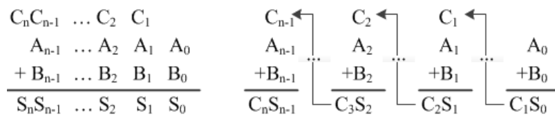
Fig. 4. N-bit ripple-carry adder with operation format and ripple carry effect
