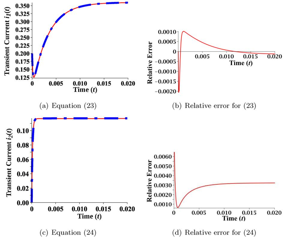
**Fig. 3.** Numerical solution of  $i_1$  (16) and  $i_2$  (17) (dash-dot) against approximate solutions (continuous line) (23) and (24), respectively. Time is in seconds and current in Amperes.
