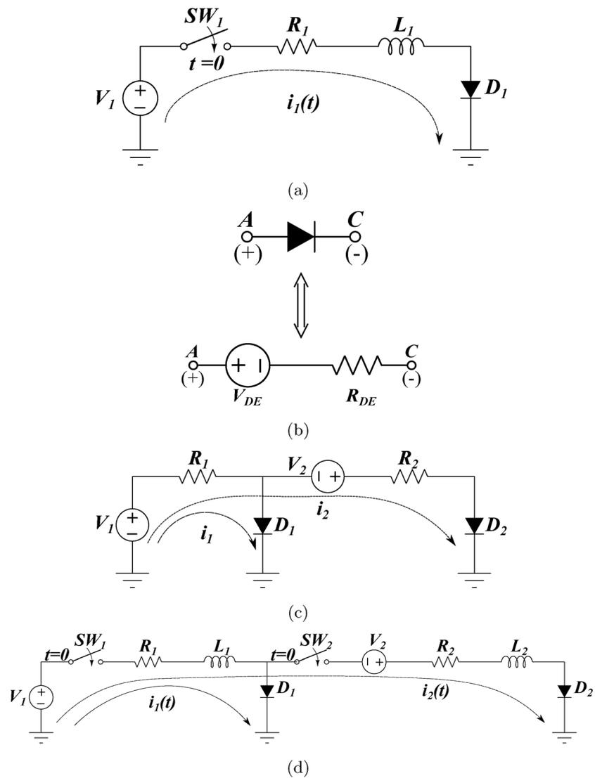
**Fig. 1.** a) Basic cell, b) Proposed equivalent diode model, c) DC scheme of two mesh circuit, and d) Transient scheme of two mesh circuit.
