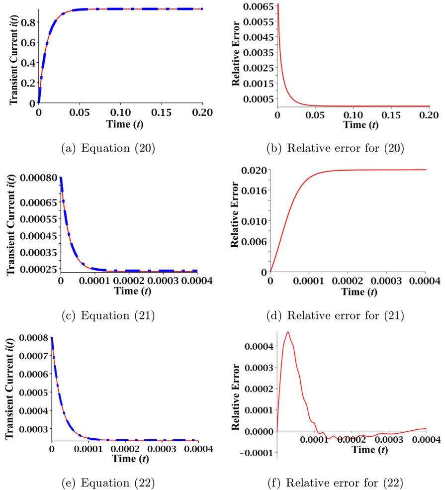
**Fig. 2.** Numerical solution for (2) (dash-dot) against approximate solution (continuous line) (20), (21) and (22). Time is in seconds and current in Amperes.
