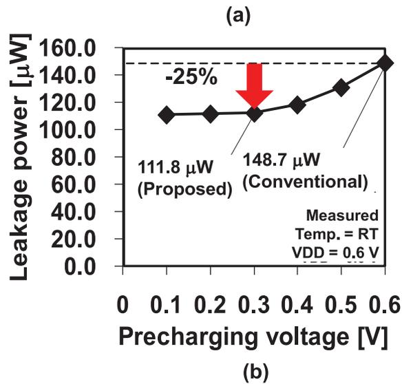
Fig. 3. (a) Shmoo plot and (b) measured leakage power in the proposed DW8T SRAM when a precharging voltage is changed.
