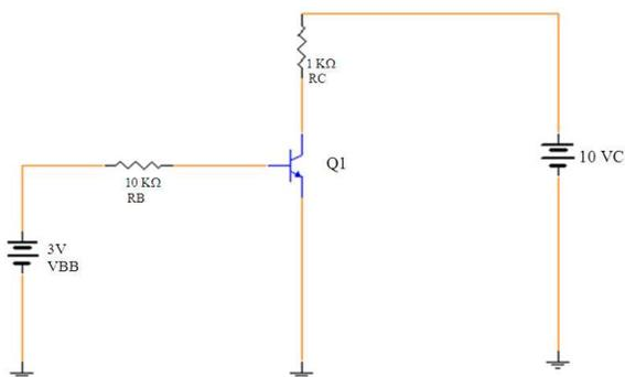
Fig. 6: standard bias circuit
