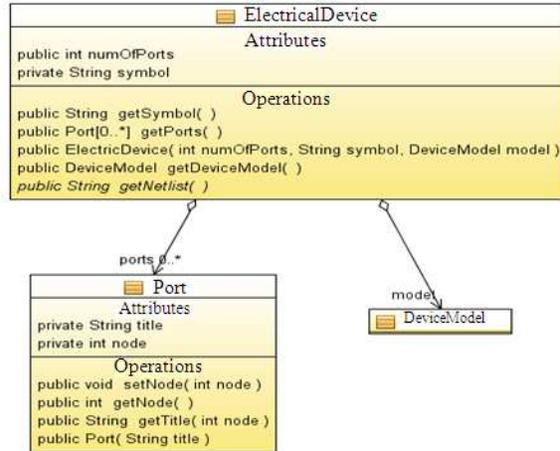
Fig. 1: Class ElectricDevice
