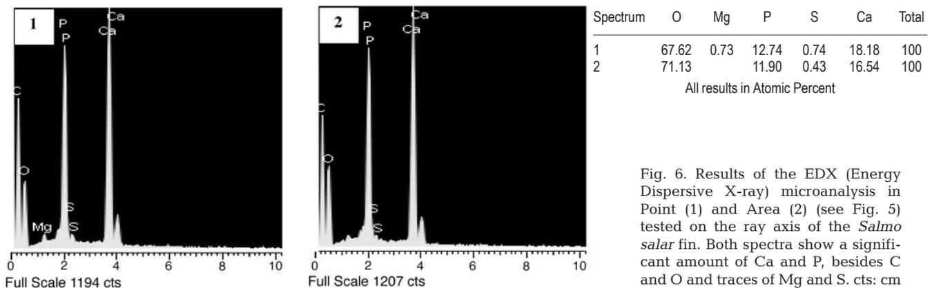
Fig. 6. Results of the EDX (Energy Dispersive X-ray) microanalysis in Point (1) and Area (2) (see Fig. 5) tested on the ray axis of the *Salmo salar* fin. Both spectra show a significant amount of Ca and P, besides C and O and traces of Mg and S. cts: cm
