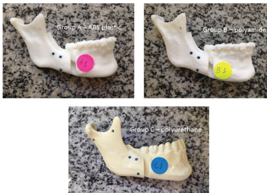
Fig. 3 Samples of Groups A, B, and C fixated with inverted L screws.
