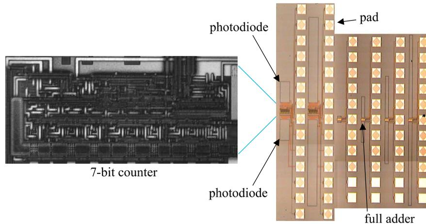
Fig. 2. Micrograph of test chip
