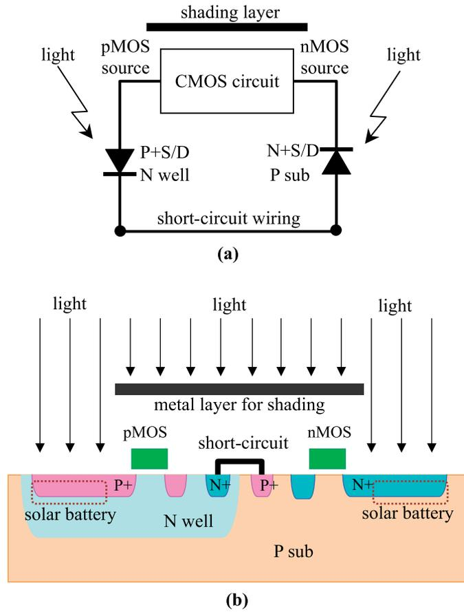
Fig. 1. Structure of on-chip solar battery: (a) equivalent circuit structure (b) section structure of device
