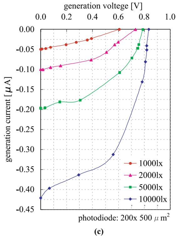
**Fig. 3.** Evaluation results: (a) drive performance for full adder (b) drive performance for 7-bit counter (c) I-V characteristic of proposed solar battery
