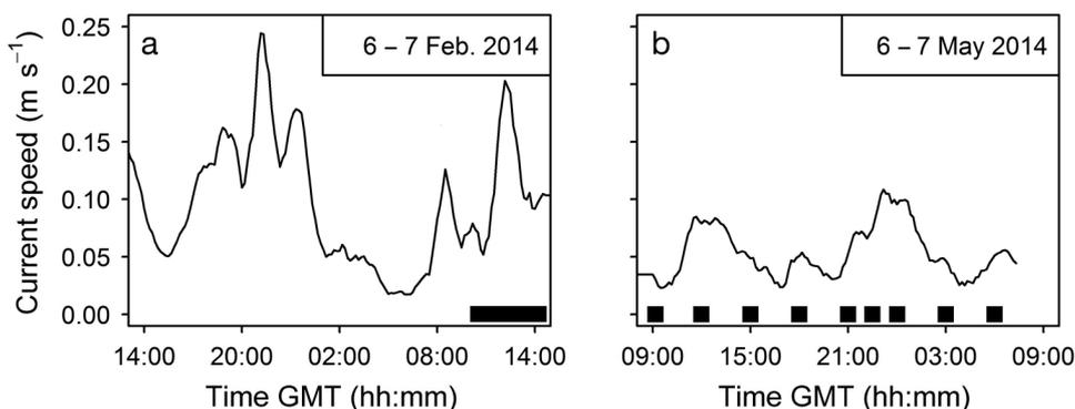
Fig. 2. Current speed (smoothed 1 h running average) at 1 m depth at (a) the spatial and (b) the temporal survey sites. The current meter was closer to the shore at the temporal survey site (see Fig. 1). The black bar in (a) denotes the sampling period for the spatial sampling, and black squares in (b) represent the tim-
