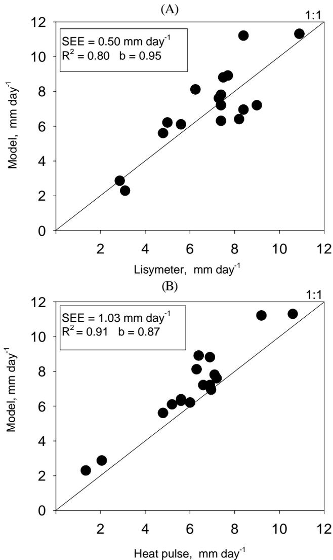
Figure 5. Relationship between estimated transpiration and measured water uptake of maize by lysimeter (A) and heat pulse technique (B), during the growing season of 1996/1997. Results from regression analysis and standard error of estimate (SEE) are shown
