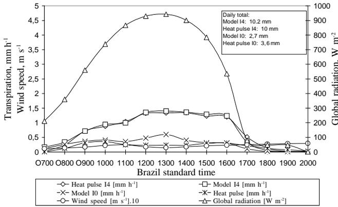
Figure 2. Hourly and daily estimated transpiration and measured water uptake by heat pulse technique, in maize, during non-stress (I4) and severe stress conditions (I0), with high evaporative atmospheric demand, on 12/16/1995
