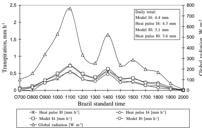
Figure 3. Hourly and daily estimated transpiration and measured water uptake by heat pulse technique, in maize, during non-stress (I4) and severe stress conditions (I0), with low evaporative atmospheric demand, on 01/09/1997
