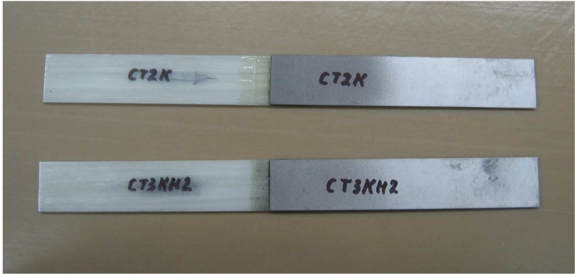
Fig. 5. Photo image of samples for testing adhesive bonds of fiberglass and titanium alloy elements
