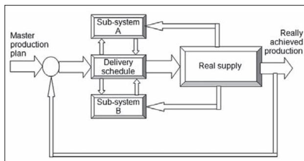
**Figure 5** Concept of hybrid decision support system for iron ore supply
