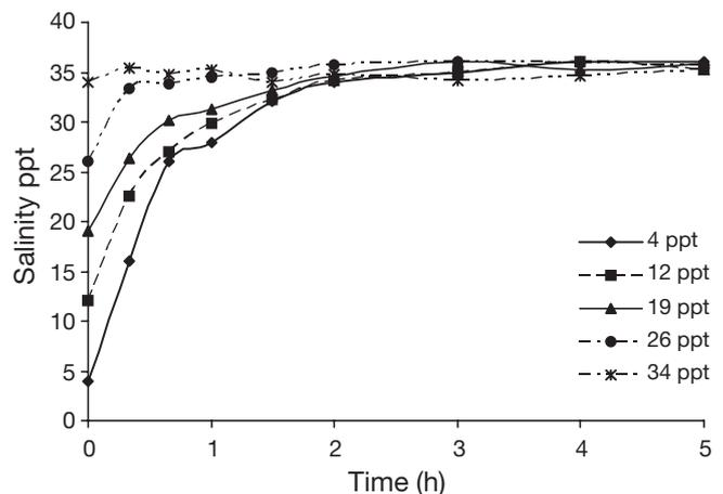
Fig. 1. Change in salinity profile over time after tank inflow had been switched to full strength (36 ppt) seawater
