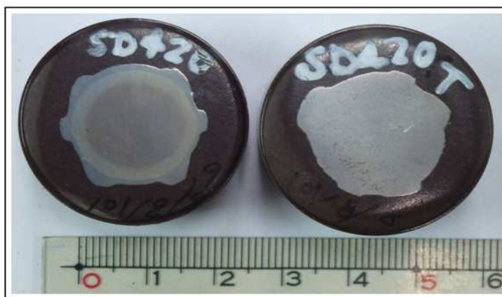
Fig. 1. Etched specimens (left: Heat-treated steel; right: Hot-rolled steel)
