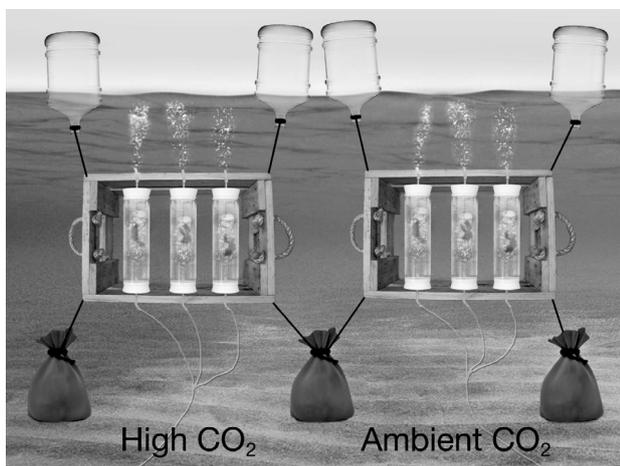
Fig. 1. Experimental design: cylinders were fixed using a wooden frame
